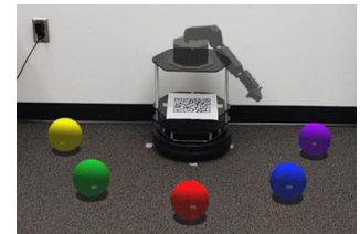
(d) Physical Robot with a virtual (AR) arm pointing to a virtual (AR) referent (V→V)
