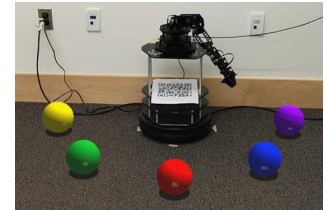
(b) Physical Robot with a physical arm pointing to a virtual (AR) referent (P→V)
