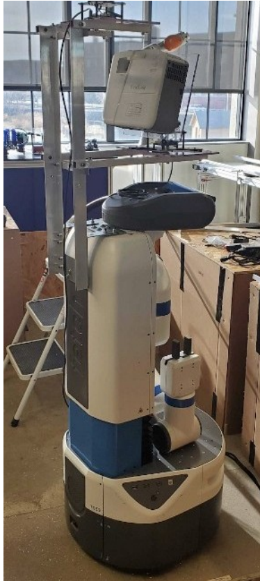
Figure 36: A sample use, where a projector is mounted onto a Fetch robot via a custom hardware structure attached to its upper back and a turret unit to pan and tilt the projector. However, the projection mapping technique is robot agnostic and the projector does not have to be attached to the robot. See Section 5.7 for more details.
