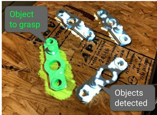
Figure 33: The projection of perception results: the detected objects (white and green) and the object to be manipulated (green). Using our implementation of projection mapping, researchers and practitioners can enable a robot to accurately externalize internal states for explanation. A video is available at https://youtu.be/S0z9e2gUrEA .
