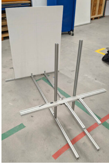
Figure 35: We calculated the intrinsics of our particular projector by mounting it perpendicular to a posterboard at a fixed distance. See Section 5.4 for more details.
